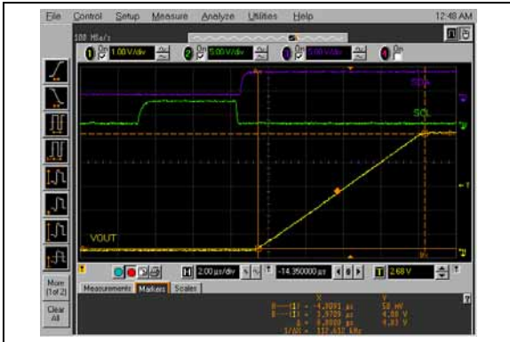
FIGURE 2-96: Full-Scale Settling Time (000h to FFFh) (MCP4726).
