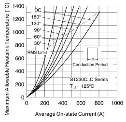
Fig. 6 - On-State Power Loss Characteristics
