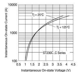
Fig. 9 - On-State Voltage Drop Characteristics
