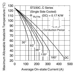
Fig. 2 - Current Ratings Characteristics
