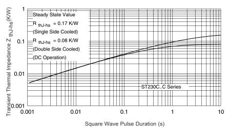
Fig. 10 - Thermal Impedance Z<sub>thJ-hs</sub> Characteristics
