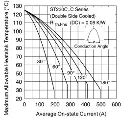
Fig. 3 - Current Ratings Characteristics
