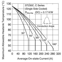
Fig. 1 - Current Ratings Characteristics
