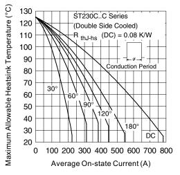
Fig. 4 - Current Ratings Characteristics
