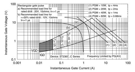
Fig. 11 - Gate Characteristics
