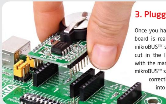
Once you have soldered the headers your board is ready to be placed into desired mikroBUS™ socket. Make sure to align the cut in the lower-right part of the board with the markings on the silkscreen at the mikroBUS™ socket. If all the pins are aligned correctly, push the board all the way into the socket.
