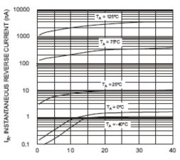
V<sub>R</sub>, INSTANTANEOUS REVERSE VOLTAGE (V) Fig. 2 Typical Reverse Characteristics
