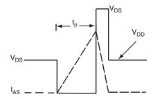
Fig. 15 - Unclamped Inductive Waveforms
