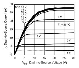
Fig. 1 - Typical Output Characteristics
