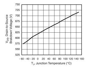
Fig. 10 - Temperature vs. Drain-to-Source Voltage
