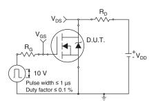
Fig. 12 - Switching Time Test Circuit
