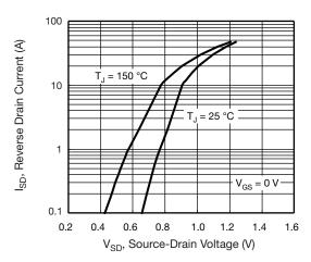
Fig. 7 - Typical Source-Drain Diode Forward Voltage
