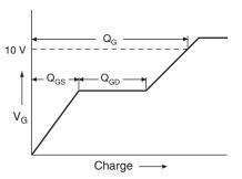
Fig. 16 - Basic Gate Charge Waveform
