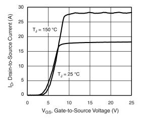
Fig. 3 - Typical Transfer Characteristics
