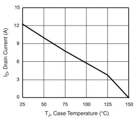
Fig. 9 - Maximum Drain Current vs. Case Temperature
