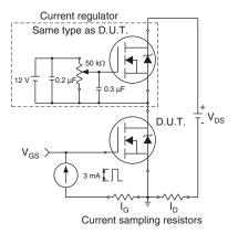
Fig. 17 - Gate Charge Test Circuit
