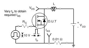
Fig. 14 - Unclamped Inductive Test Circuit
