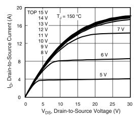
Fig. 2 - Typical Output Characteristics
