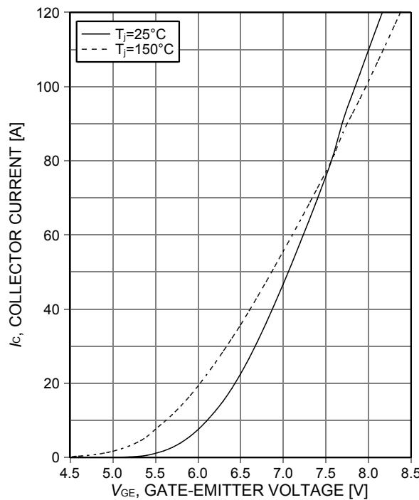
**Figure 6. Typical transfer characteristic**
