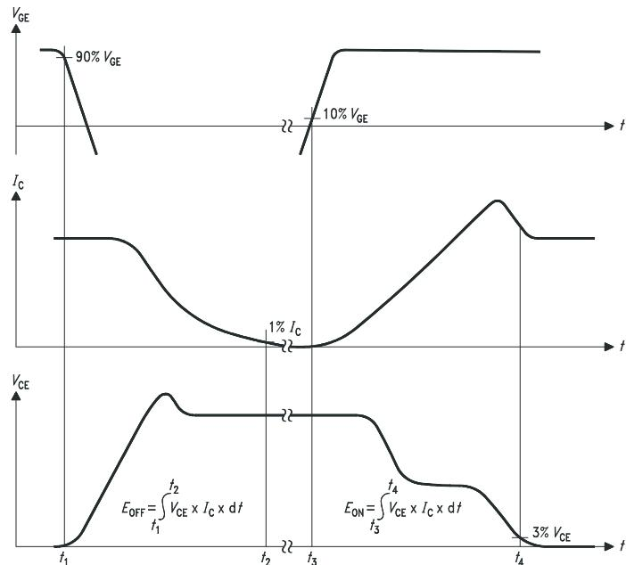
Figure B. Definition of switching losses
