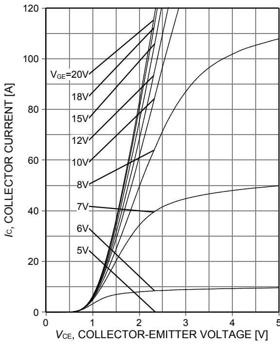
**Figure 4. Typical output characteristic**
