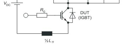
Figure E. Dynamic test circuit
