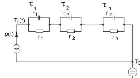
Figure D. Thermal equivalent circuit
