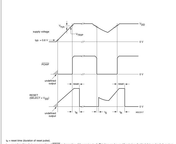
$t_S$  = save time (time between assertion of  $\overline{\mathsf{POWF}}$  and assertion of the reset output). This time can be used for storing of critical data and orderly system shut-down.
