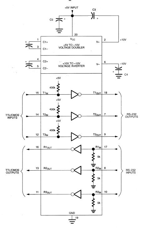
NOTE: C5 is a recommended decoupling capacitor which is the same value as C1, C2, C3, and C4.
