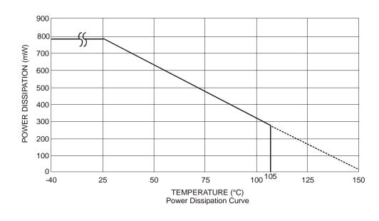
Notes: 10. U-DFN2020C-6 exposed pad soldered to minimum recommended landing pads (see Package Outline Dimension section) on a two-layer 2oz. copper FR4 PCB (1.6mm thickness) with no thermal vias in exposed PADs or any copper flood connecting to the landing pattern of the exposed pad.
