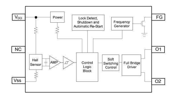
Notes: 2.The AH5794 has an open-drain tachometer FG output that follows the magnetic change frequency. Typically a pull-up resistor of 10kΩ is recommended from FG pin to the supply voltage.
