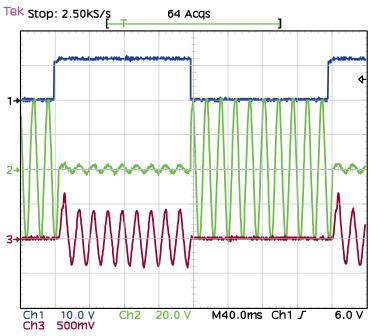
**Channel 1:** EN signal 0 to 12V logic input turning the solenoid on and off.
