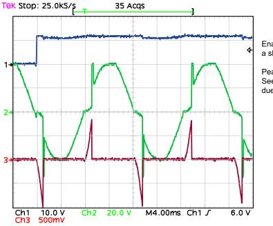
Enable from low to high into a shorted solenoid.
