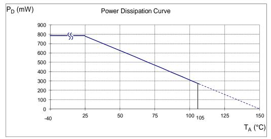
11. DFN2020C-6 exposed pad soldered to minimum recommended landing pads (see Package Outline Dimension section) on a two-layer 2oz. copper FR4 PCB (1.6mm thickness) with no thermal vias in exposed PADs or any copper flood connecting to the landing pattern of the Notes: exposed pad.
