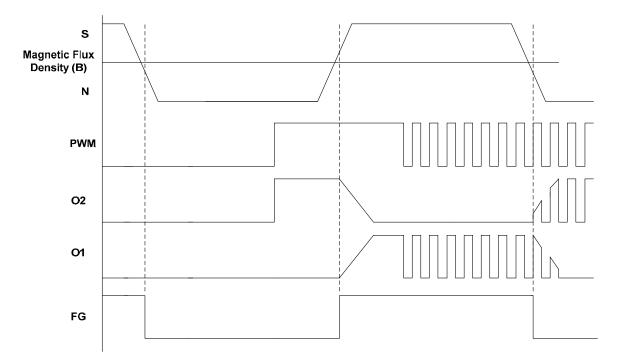
Frequency of PWM speed control signal can be between 15Hz to 50kHz. Recommended typical PWM signal frequency is 25kHz to keep switching frequency away from audible band. If PWM signal level at PWM pin stays low for longer than 65ms typical, the outputs are disabled.
