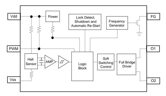
Notes: 3. The AH5795 has an open-drain tachometer FG output that follows the magnetic change frequency. Typically a pull-up resistor of 10KΩ is recommended from FG pin to the supply voltage.
