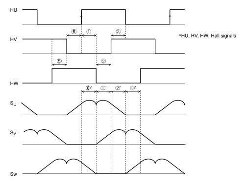
In the above diagram, the modulated waveforms have an interval ①') equal to the interval of 1/32 between a rising edge of HU to a falling edge of HW (①). And the modulated waveforms have an interval (②') equal to the interval of 1/32 between a falling edge of HW to a rising edge of HV (②). If there is not an HU rising edge before 32 ticks ends, ②' becomes equal to ①' until the next rising edge of HU.
