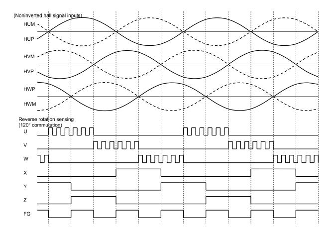
\*: When CW/CCW = High, noninverted Hall signals put the TB6584AFNG in 120° commutation mode with a lead angle of 0° (reverse rotation).
