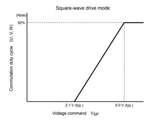
Note: The conduction period is reduced by the dead time. (carrier\_frequency  $\times$  92% - T<sub>D</sub>  $\times$  2)
