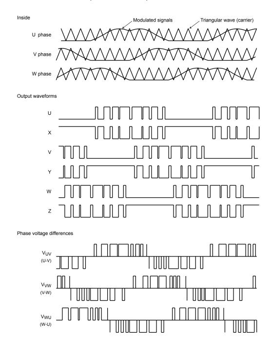
In sine-wave drive mode, the amplitude of the modulated signals varies with the VSP voltage, and the motor speed changes with the conduction duty cycle of the output waveforms. (See the sine-wave drive mode diagram on page 13.)
