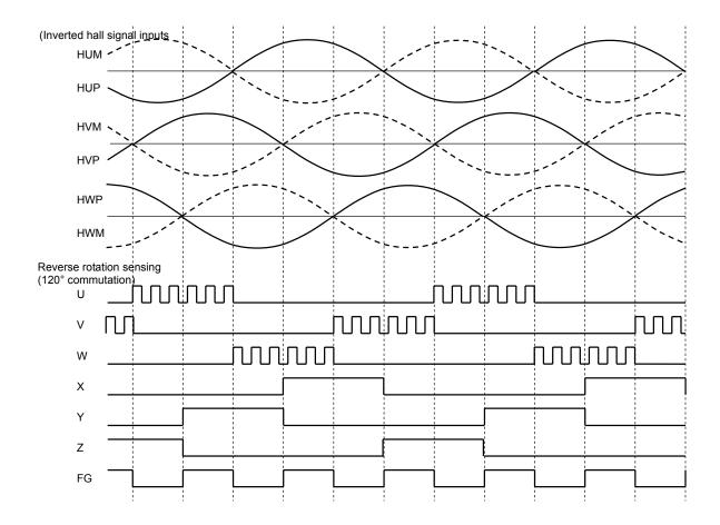
\*: When CW/CCW = Low, inverted Hall signals put the TB6584AFNG in 120 commutation mode with a lead angle of 0° (reverse rotation).
