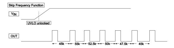
Switching frequency is changed as follows. ...  $\times 0.9 \rightarrow \times 1.1 \rightarrow \times 1.05 \rightarrow \times 1 \rightarrow \times 0.95 \rightarrow \times 0.9 \rightarrow \times 1.1$  ... It's repeated by this loop.
