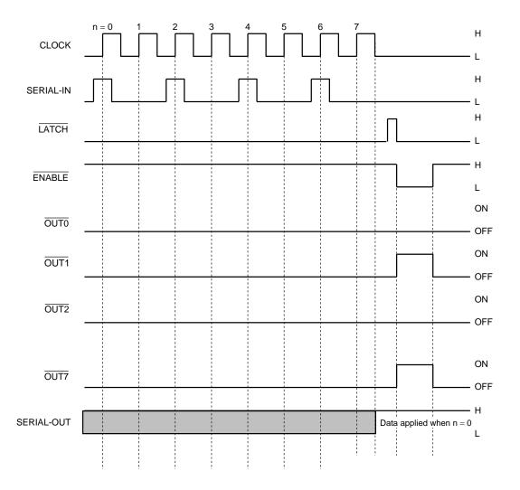
Note 1: Latches are level-sensitive, not edge-triggered.
