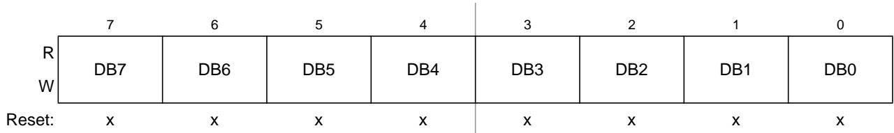
Figure 12-33. Data Segment Registers (DSR0–DSR7) — Extended Identifier Mapping
