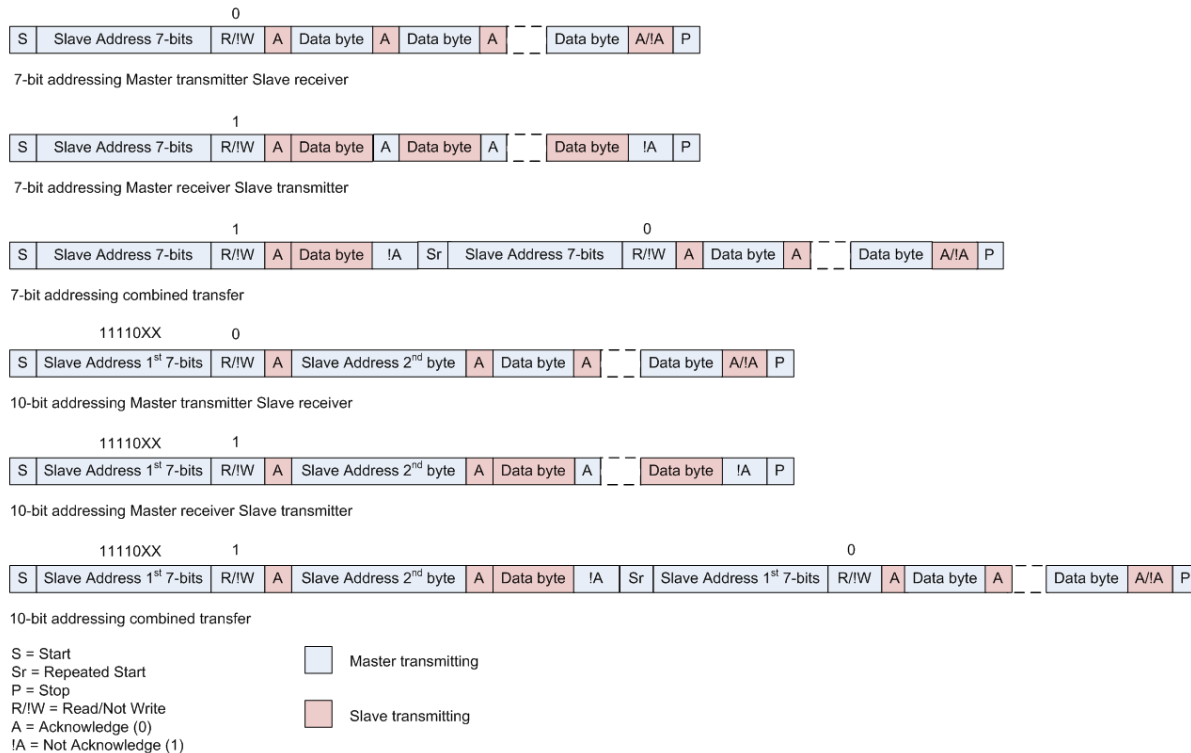
Figure 9.2: Data transfers with 7-bit and 10-bit addressing modes
