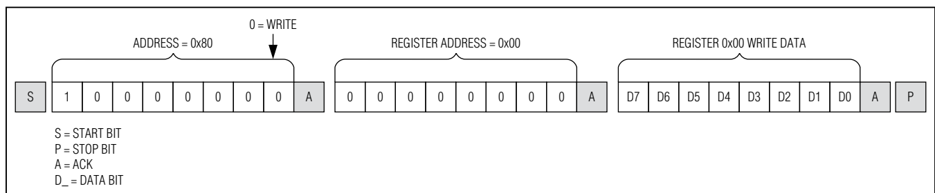
Figure 26. Format for I 2 C Write
