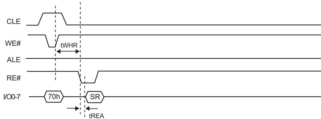
Figure 6.24 Read Status Timing
