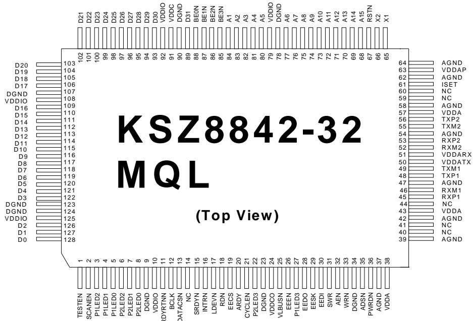
Figure 5. Standard – KSZ8842-32 MQL 128-Pin PQFP (Top View)
