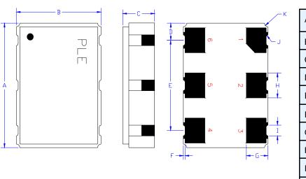
Gold 11.8  $\mu inches$  0.3  $\mu m$  minimum over Nickel 50 to 350  $\mu inches$  1.27 to 8.89  $\mu m$
