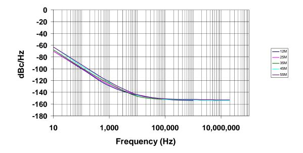
Typical phase noise plot for 5 oscillators at different output frequencies.
