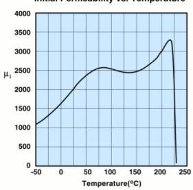
Measured on an 18/10/6mm toroid at 100kHz.
