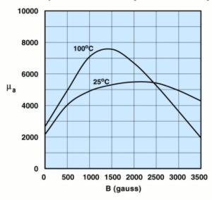
Measured on an 18/10/6mm toroid at 10kHz.
