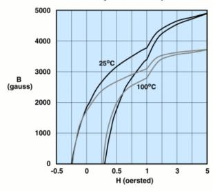
Measured on an 18/10/6mm toroid at 10kHz.
