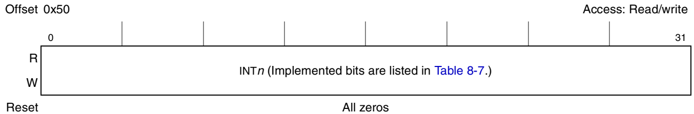
Figure 8-19. System Internal Interrupt Force Register (SIFCR_H)
