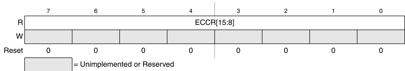
Figure 25-20. Flash ECC Error Results High Register (FECCRHI)
