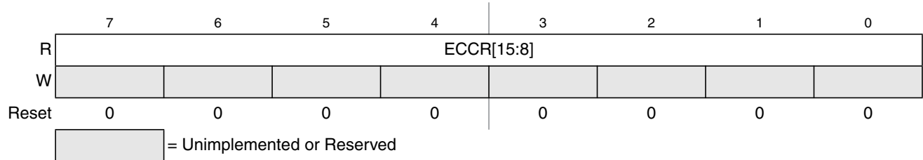
Figure 26-20. Flash ECC Error Results High Register (FECCRHI)
