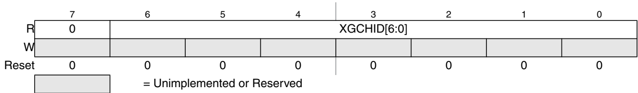
Figure 10-4. XGATE Channel ID Register (XGCHID)
