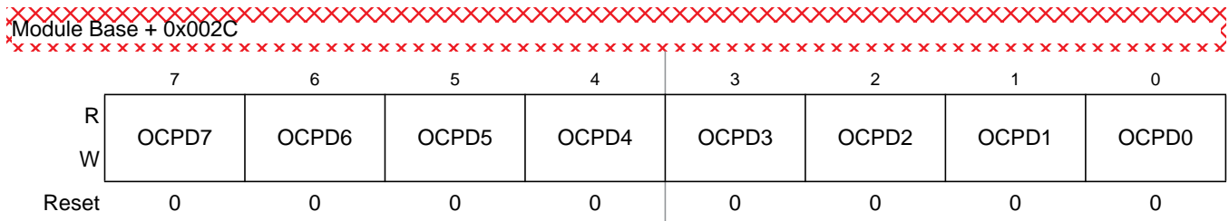
Figure 14-28. Output Compare Pin Disconnect Register (OCPD)
