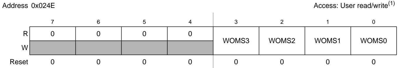
Figure 2-28. Port S Wired-Or Mode Register (WOMS)
