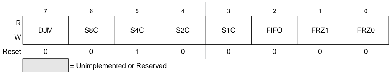
Figure 9-6. ATD Control Register 3 (ATDCTL3)
