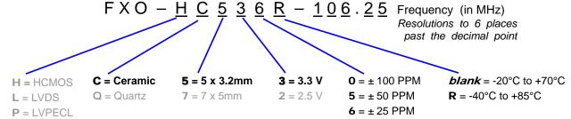
$8 = \pm 20 \text{ PPM } (-20 \sim +70^{\circ}\text{C})$
