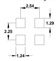
Note: XPRESSO HCMOS XOs are designed to fit on industry standard, 4 pad, layouts.
