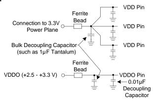
All power supply pins must be connected to the same voltage, except VDDO, which may be connected to a lower voltage in order to change the output level.
