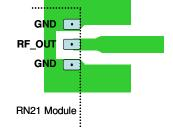
Recommended on-chip antenna is Yageo SMT high performance chip for Bluetooth/802.11b/g 2.45GHz (3.6mm x 7.2mm)
