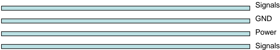
Figure 5: Typical 4-layer PCB construction
