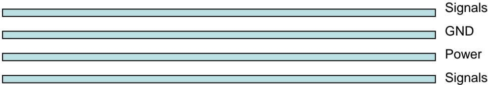
Figure 14: Typical 4-layer PCB construction
