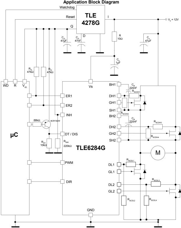
This application block diagram shows one of the possibilities to use this Driver IC. The voltage divider networks accross the 4 MOSFETs (resistors  $R_{\text{SCDLx}}$ ) allow to increase the current limit threshold for Short Circuit protection. The  $R_{\text{SCDLx}}$  resistors also provide a charge path for the bootstrap capacitors. If  $R_{\text{SCDLx}}$  resistors are not used in the application, a 12k Ohm resistor should be introduced between SH1 to GND and SH2 to GND.
