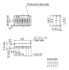
Unless otherwise specified, tolerance :  $\pm$  0.3 (Unit : mm)
