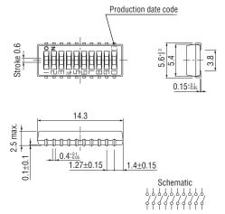
Unless otherwise specified, tolerance :  $\pm$  0.3 (Unit : mm)
