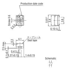
Unless otherwise specified, tolerance :  $\pm$  0.3 (Unit : mm)
