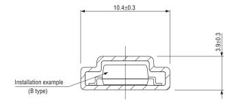
\*The magazine is common to A and B terminal pin.
