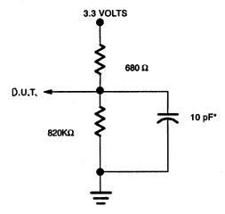
\* INCLUDING SCOPE AND JIG CAPACITANCE
