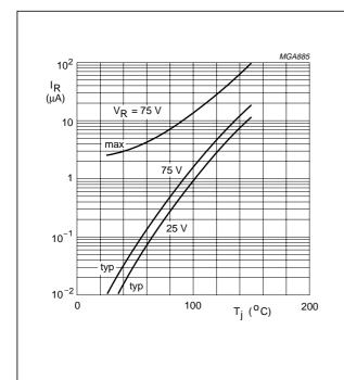
Fig.5 Reverse current as a function of junction temperature.
