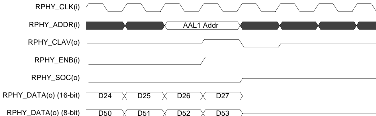
Figure 90 UI_SRC_INTF End-of-Transfer Timing (Utopia 2 PHY Mode)
