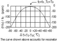
contribution only and does not include LC component temperature characteristics.
