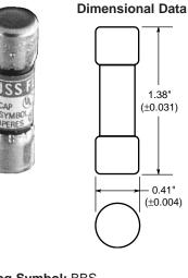
Catalog Symbol: BBS Fast-Acting 1/10 TO 30A Interrupting Rating: 10 KA UL Listed, STD. 248-14 0-5A/600Vac OR LESS, 6-10A/250Vac (GUIDE #JDYX, FILE #E19180) CSA CERTIFIED, C22.2 NO. 248.14 0-5A/600V, 6-10A/250Vac (CLASS #1422-01, FILE #53787)
