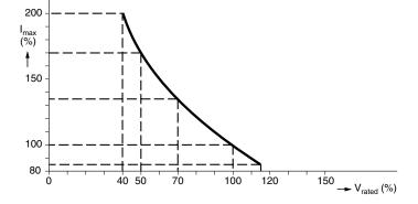
$I_{max}$  as stated in the Electrical data and ordering information tables, is the maximum overload current that may flow through the PTC when passing from the low ohmic to high ohmic state at rated voltage.
