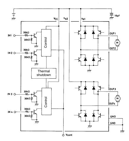
Note: As long as the voltages applied to  $V_{CC}$ ,  $V_S1$ ,  $V_S2$ , and IN1 through IN4 are within the limits set by the absolute maximum ratings, there are no restrictions on the relationship of each voltage level in comparison with the others (regarding which is higher or lower). (ex.  $V_{CC} = 3 V$ ,  $V_S1$ , 2 = 2 V, IN1 to IN4 = 5 V)
