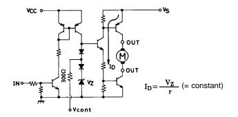
As shown in the above diagram, the Vcont pin outputs the voltage of the band gap Zener  $V_Z+V_F$  (= 1.93 V). In normal use, this pin is left open. The drive current  $I_D$  is varied by the Vcont voltage. However, because the band gap Zener is shared, it functions as a bridge.
