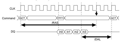
Note: Internal auto-precharge starts at the timing indicated by " \ ". and an interval of tRAS (IRAS) is required between previous active (ACT) command and internal precharge " \ ".
