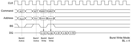
WRITE to WRITE Command Interval (different bank)
