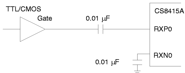
Figure 17. TTL/CMOS Input Circuit
