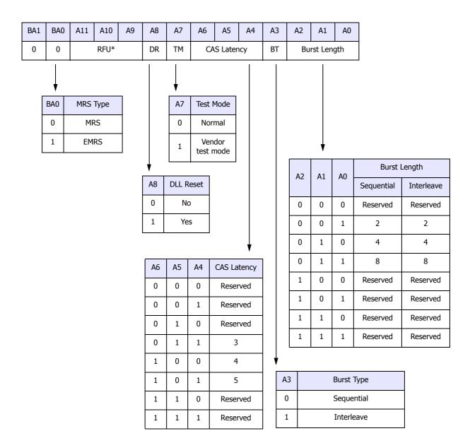
\* All bits in RFU address fields must be programmed to Zero, all other states are reserved for future usage. And, if MRS/EMRS are programmed with 'Reserved' code, it could be the cause of mal-function.
