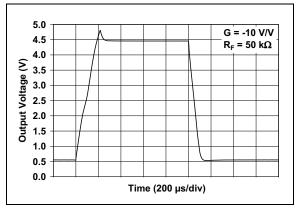
**FIGURE 2-34:** Large Signal Inverting Pulse Response vs. Time.
