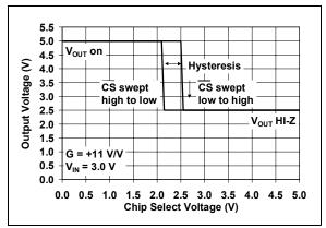
**FIGURE 2-35:** Output Voltage vs. Chip Select (CS) Voltage (MCP6143 only).
