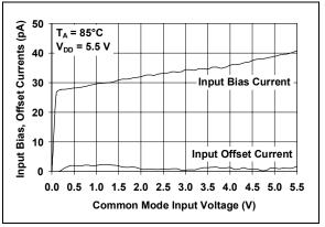
**FIGURE 2-10:** Input Bias, Offset Currents vs. Common Mode Input Voltage with Temperature = 85°C.
