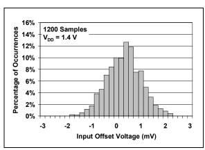
**FIGURE 2-2:** Histogram of Input Offset Voltage with  $V_{DD} = 1.4V$ .
