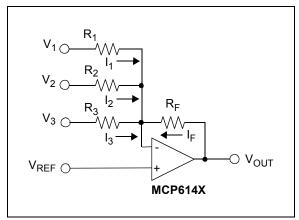
FIGURE 3-10: Summing amplifier circuit.
