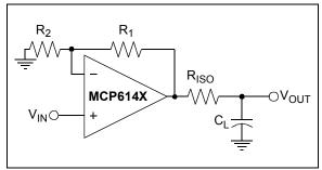
**FIGURE 3-4:** Amplifier circuit for heavy capacitive loads.
