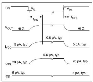
**FIGURE 3-5:** Timing Diagram for the  $\overline{CS}$  function on the MCP6143 op amp.
