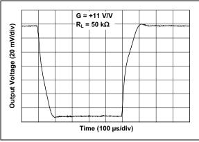
**FIGURE 2-27:** Small Signal Non-Inverting Pulse Response vs. Time.
