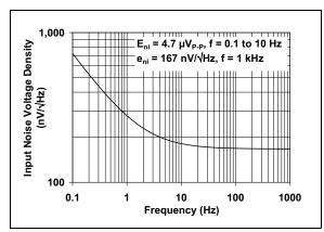
**FIGURE 2-8:** Input Noise Voltage Density vs. Frequency.
