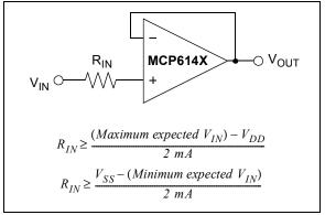
**FIGURE 3-1:** An input resistor, R<sub>IN</sub>, should be used to limit excessive input current if the inputs exceed the absolute maximum specification.
