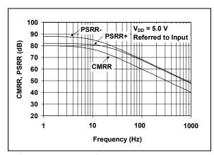
**FIGURE 2-9:** Common Mode Rejection Ratio, Power Supply Rejection Ratio vs. Frequency.
