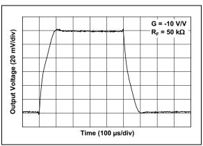
**FIGURE 2-30:** Small Signal Inverting Pulse Response vs. Time.
