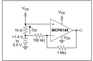
FIGURE 3-9: High Side Battery Current Sensor.
