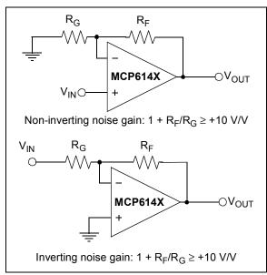
**FIGURE 3-2:** Noise gain for inverting and non-inverting amplifier configuration.
