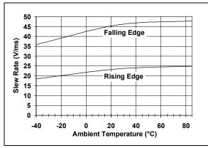
FIGURE 2-25: Slew Rate vs. Ambient Temperature.
