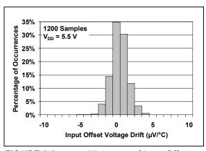
**FIGURE 2-3:** Histogram of Input Offset Voltage Drift with  $V_{DD} = 5.5V$ .
