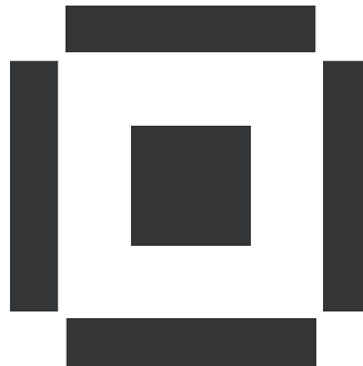
Figure 78. 82574 Silkscreen and Components Pad (Top View)
