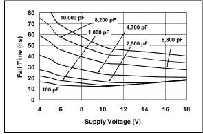
**FIGURE 2-4:** Fall Time vs. Supply Voltage.
