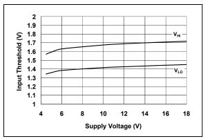
FIGURE 2-11: Input Threshold vs. Supply Voltage.
