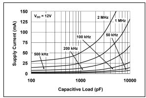
FIGURE 2-14: Supply Current vs. Capacitive Load.
