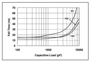
FIGURE 2-5: Fall Time vs. Capacitive Load.
