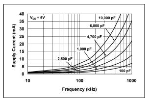
**FIGURE 2-18:** Supply Current vs. Frequency.
