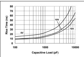
FIGURE 2-2: Rise Time vs. Capacitive Load.
