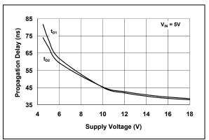
**FIGURE 2-6:** Propagation Delay vs. Supply Voltage.
