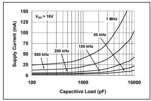
FIGURE 2-13: Supply Current vs. Capacitive Load.
