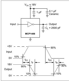
**FIGURE 4-1:** Inverting Driver Timing Waveform.
