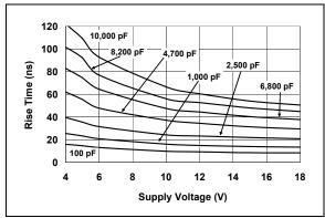
**FIGURE 2-1:** Rise Time vs. Supply Voltage.
