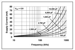
**FIGURE 2-17:** Supply Current vs. Frequency.
