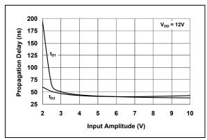
**FIGURE 2-7:** Propagation Delay Time vs. Input Amplitude.
