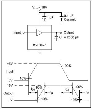
FIGURE 4-2: Non-Inverting Driver Timing Waveform.
