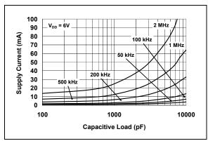
FIGURE 2-15: Supply Current vs. Capacitive Load.
