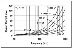
**FIGURE 2-16:** Supply Current vs. Frequency.
