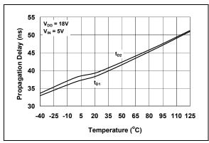
**FIGURE 2-8:** Propagation Delay Time vs. Temperature.
