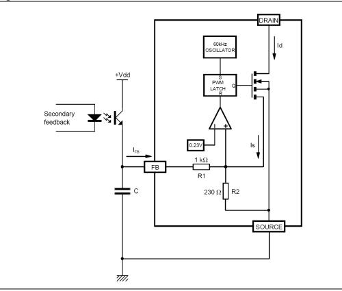
Figure 4. Internal current control structure
