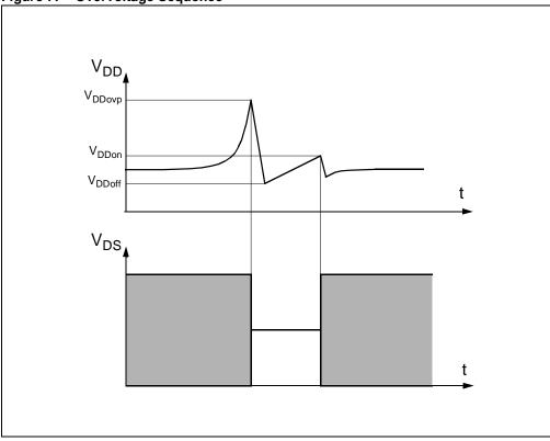
Figure 7. Overvoltage Sequence
