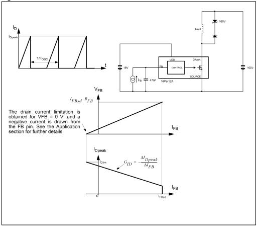
Figure 11. Peak drain current Vs. feedback current
