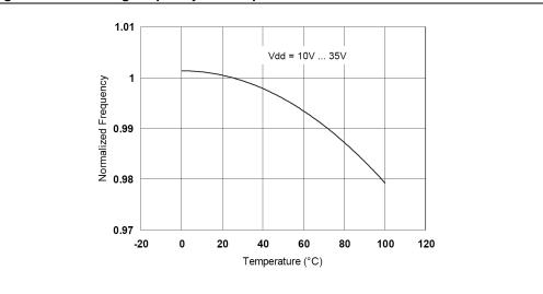
Figure 13. Switching frequency Vs. temperature
