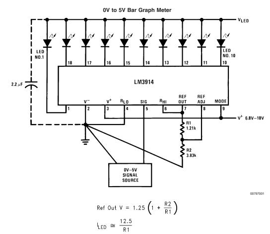
Note: Grounding method is typical of all uses. The 2.2µF tantalum or 10 µF aluminum electrolytic capacitor is needed if leads to the LED supply are 6" or longer.
