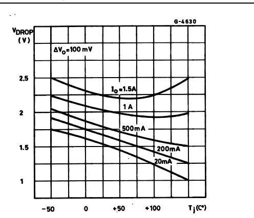
**Figure 5.** Reference voltage vs junction
