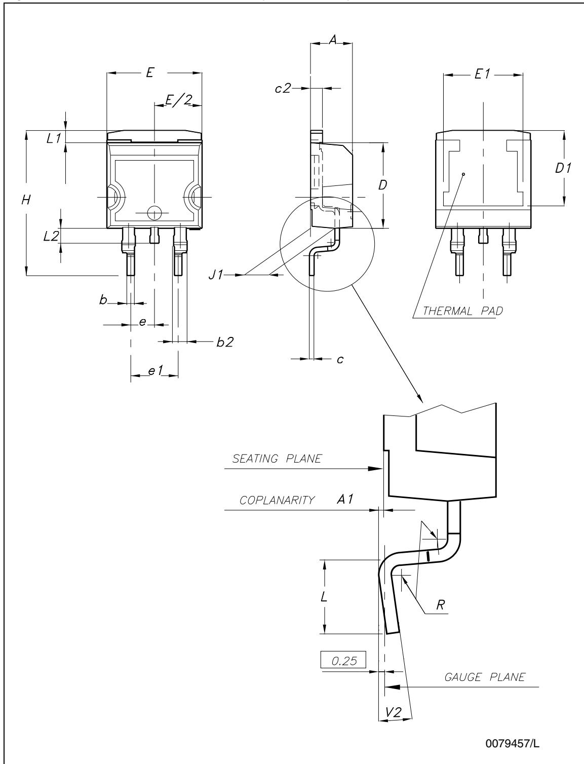
**Figure 15. DRAWING DIMENSION D<sup>2</sup>PAK (TYPE WOOSEOK-SUBCON.)**
