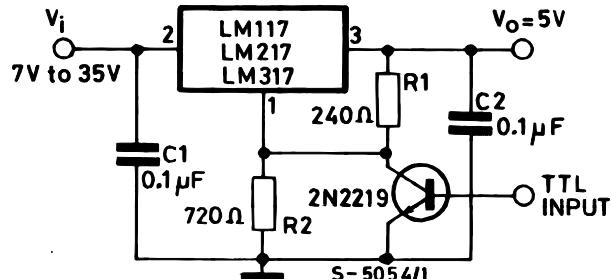
**Figure 11. Digitally selected outputs**
