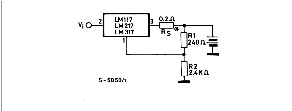
\*  $R_S$  sets output impedance of charger  $Z_O = R_S (1 + R_2/R_1)$ . Use of  $R_S$  allows low charging rates with fully charged battery.
