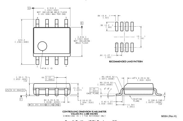
Small Outline (SO) Package (M) Order Number LM236M-2.5, LM236AM-2.5, LM336M-2.5 or LM336BM-2.5 **NS Package Number M08A**
