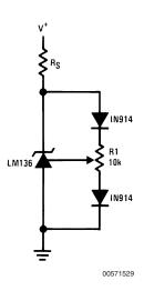
FIGURE 2. Temperature Coefficient Adjustment (Trim Range = ±70 mV typical)
