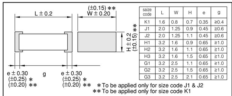
■ Taping Specification for Automatic Mounting
