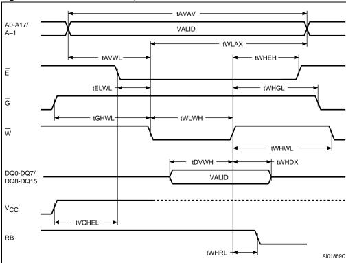
Figure 9. Write AC waveforms, Write Enable controlled
