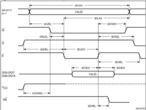
Figure 10. Write AC waveforms, Chip Enable controlled
