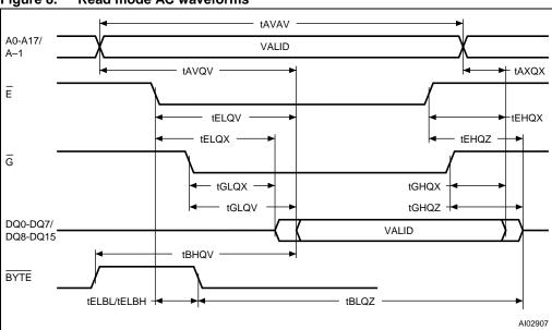
Figure 8. Read mode AC waveforms
